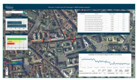
Fig. 3 - Screenshot of the Rheticus platform showing displacement monitoring over the city of Milan, Italy.
