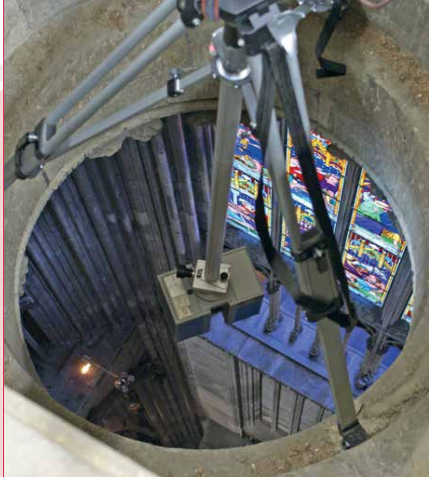
Img. 1 - The Z+F IMAGER® 5010X used head first high above the church's ground floor.
