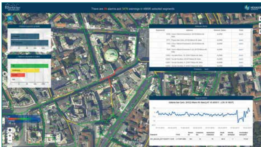
Fig. 3 - Dynamic geoinformation about displacements over the sewer Network in Milan, Italy.
