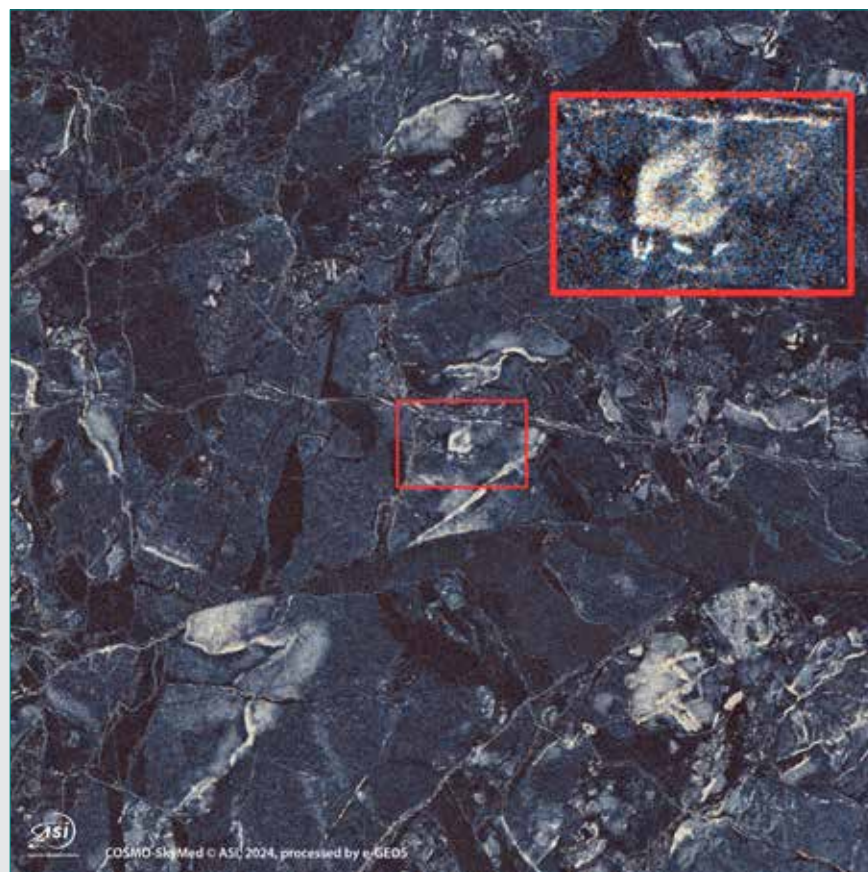
Italian COSMO-SkyMed satellite constellation collects images of vehicles parked at the northernmost point of the planet. Spotlight-2B mode (area 10km x 10km, spatial resolution 0.6m) acquired in dual polarisation (HH+HV). COSMO-SkyMed Second Generation Image © 2024 ASI. Processed by e-GEOS
