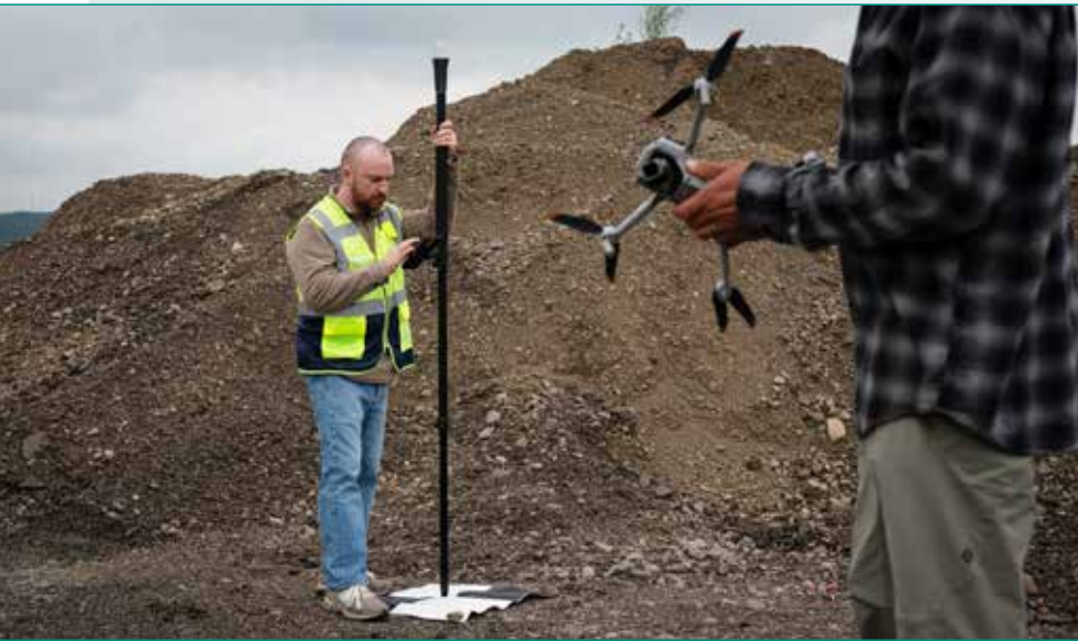
Measuring GCP with Emlid Reach RX
