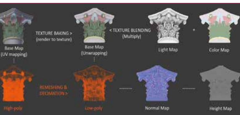
Fig. 12 - Model simplification and texture baking workflow in Blender.
