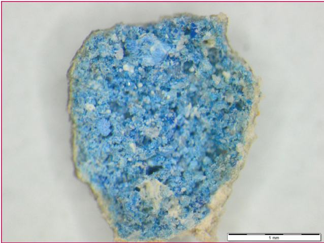
Fig. 2 - Optical photomicrograph of the blue pigment sample (microscope objective 10x)
