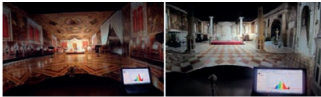
Fig. 3 - Simulated scenes as shown in a wide angle view of interior spaces created by the software using the average RGB combined with realistic textures and projected for measuring its SPD as viewed in the VR enclosure in real time.
