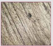
Fig.9 - ME for a sample from the group C, shows layers of lead in silver (150 X).
