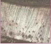
Fig. 10 - ME for cross- section of silver coins shows the islands of lead in silver (150 X).
