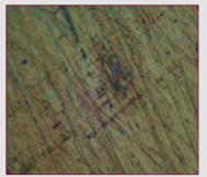
Fig.7 - ME for a sample from the group A, shows the micro crocks (50X).
